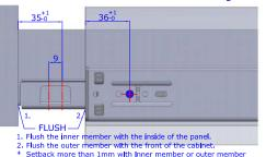
may cause damage to the soft close module when closing.
