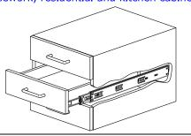
10"-14" 20mm stroke of Soft-Closing 16"-28" 36mm stroke of Soft-Closing
