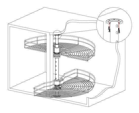
**4.** To automatically pull out the bottom basket when opening the cabinet door, attach the positioning device to the cabinet door as per below.
