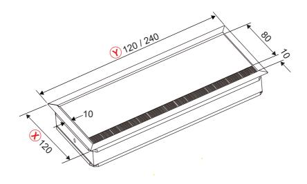
Cable passage dimension  $\bigcirc$  =  $\bigcirc$  - 36 (underside)
