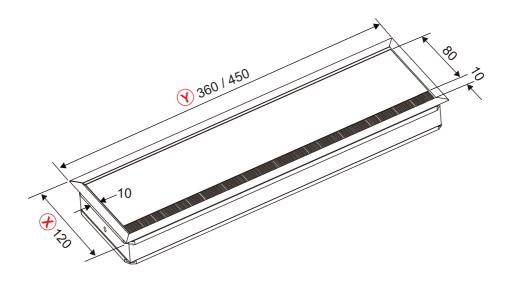
Cable passage dimension (A) = (X) - 36 (underside) (B) = (Y) - 36
