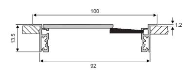
Cable passage dimension (A = X) - 32 (underside) (B = Y) - 32
