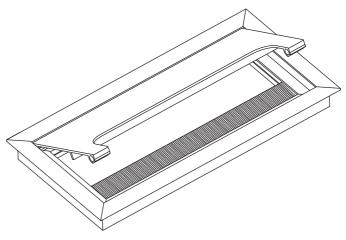
Cable passage dimension (A) = (X) - 32(underside)
