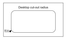
Cable passage dimension (A) = (X) - 7 (underside) (B) = (Y) - 7
